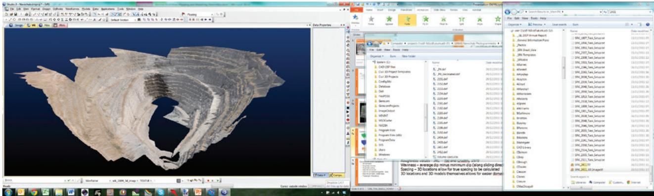
Figure 1: 3-D Mosaic image showing the hanging-wall and footwall
