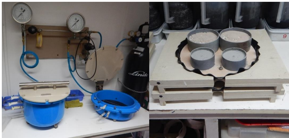
Figure 4. Pressure plate equipment used to obtain SWCC
